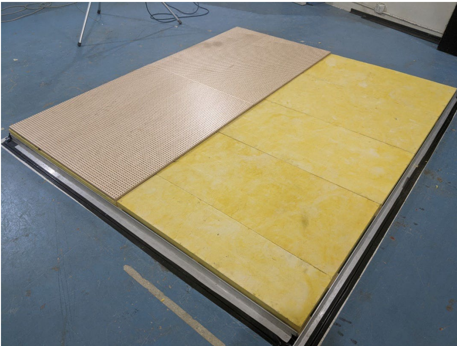
Figure 4 – Specimen panels partially installed over base layer fiberglass
